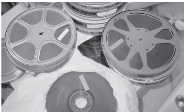
Figure 1. To test roll film in a can, place a strip on top of the film and reclose the can.
